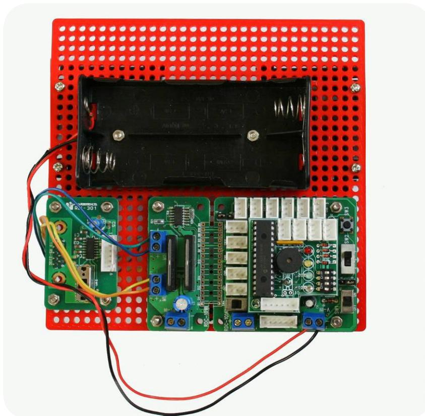
Finally, connect the serial communication board to the muvium board with the appropriate cable.
