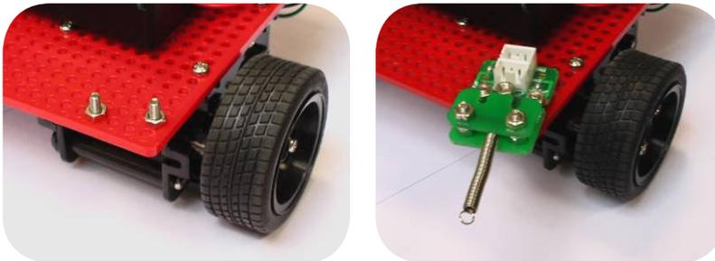
Finally, assemble both left and right touch sensors and connect with the proper cable left sensors on connector DI00 and right sensor on connector DI01 of the Muvium board as shown in the following figure.
